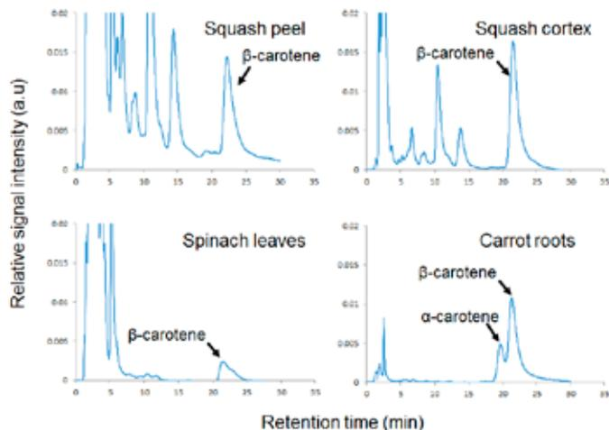
Fig. 7 - Detection of  $\alpha$ - and  $\beta$ -carotenes with HPLC. HPLC chromatograms show the peaks of carotenoids extracted with DME from squash peel, squash pericarp, spinach leaves and carrot roots. Pigments eluted from Inertsil ODS-80A column were detected by monitoring the changes in absorption at 455 nm.
