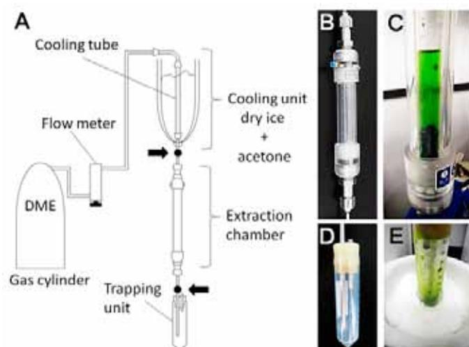
Fig. 1 - Apparatus for pigment extraction with liquefied DME. (A) Composition of the system. Arrows indicate the positions of two stopcocks for fine controls of gaseous and liquefied DME flows. (B, C) Extraction chamber. (D, E) Trapping port with a plastic tube.
