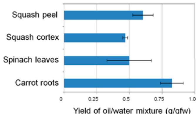
Fig. 3 - Yield of oil/water mixture extracted from vegetables using DME as solvent. Mixture of oil and water containing pigments from vegetables are compared.
