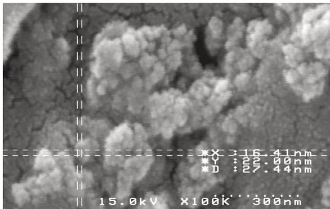
Fig. 2 - The image of magnetic nano-carboxymethylated chitosan particles by SEM microscopy. Size and morphology of Fe<sub>3</sub>O<sub>4</sub> coated by carboxymethylated chitosan.
