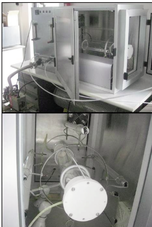
Fig. 1 - Pictures of the experimental set-up reactor for evaluating photocatalysis efficiency.
