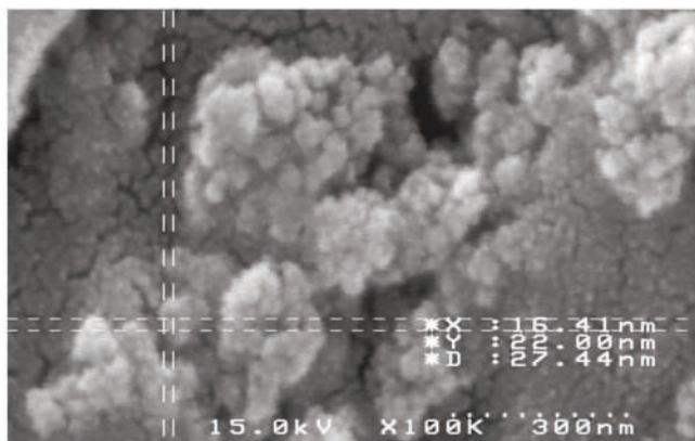
Fig. 2 - The image of magnetic nano-carboxymethylated chitosan particles by SEM microscopy. Size and morphology of Fe 3 O 4 coated by carboxymethylated chitosan.
