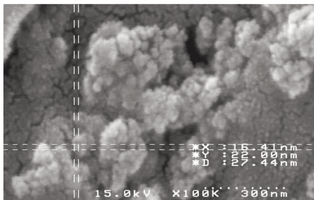
Fig. 2 - The image of magnetic nano-carboxymethylated chitosan particles by SEM microscopy. Size and morphology of \text{Fe}_3\text{O}_4 coated by carboxymethylated chitosan.
