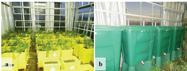
Fig. 2 - Photo of the greenhouse experiment at the University of Florence, Italy: (a) bioretention pot prototypes, (b) 200-L plastic water storage tanks.
