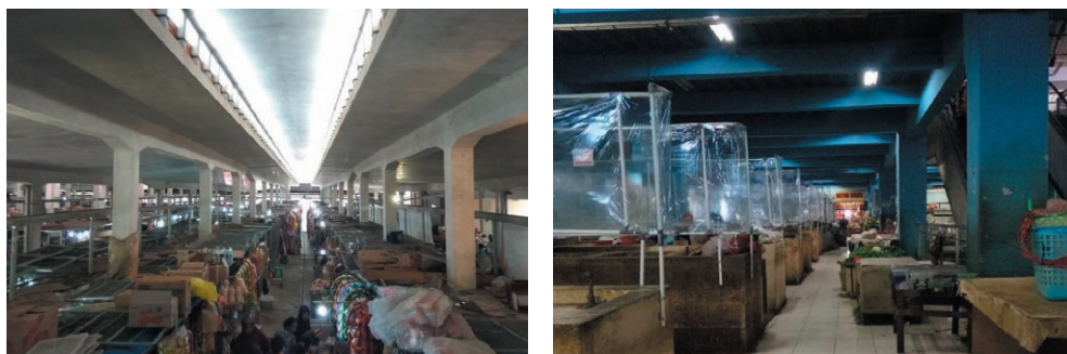
Figure 9. Peterongan Market with natural lighting (left) and Bulu Market with artificial lighting (right).
