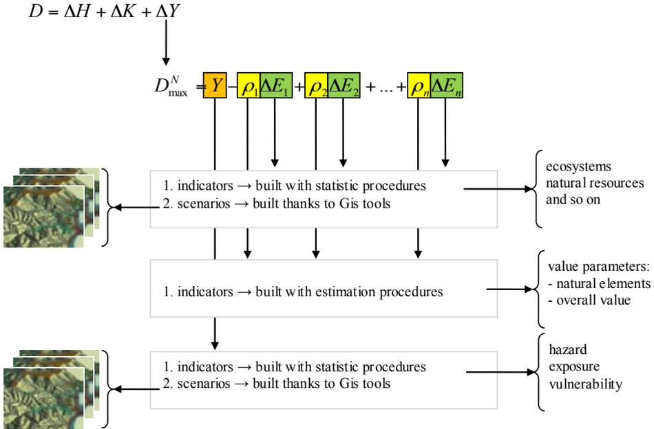
Figure 4. Scheme for the evaluation of all the elements of the damage.
