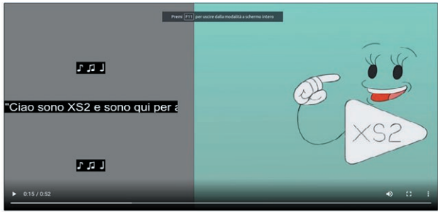
Figure 7. The incorrect implementation of position made it impossible to specify significantly long text that could wrap automatically as in the Firefox browser, forcing us to do extra work to have short sentences on spaced lines, in order for it to be correctly interpreted by the Chrome browser.
