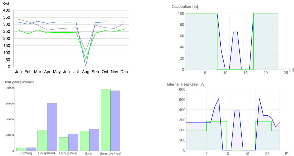
Fig. 5 Top left: Monthly electricity use (kWh) comparing standard (green), actual (grey), and billed (blue) occupant profiles. Bottom left: Energy impact of window replacement – actual (blue) vs. standard (green) profile in owned and rented units. Right: Comparison of occupancy rates (top) and internal gains (bottom) – standard (green) vs. proposed method (blue).
