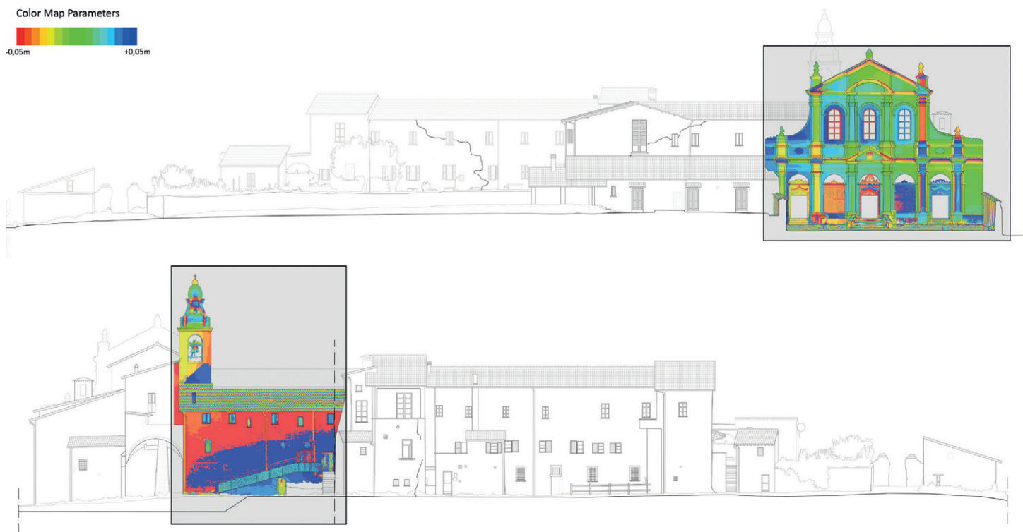
Fig. 18 Elevation maps carried out on the external walls to verify the axiality with respect to the neutral axis.
