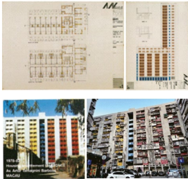
Figure 3. Red, yellow ventilation grilles and blue channels of Toi San Civilian Building Tower A (Left Photo Manuel Vicente trama e emoção = plot and emotion, P96-97. Right Photo Manuel Vicente Caressing Trivia, P152. & Photo M.Lee, 2021).
