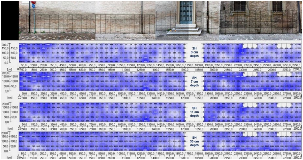
Fig. 7 Moisture maps related to the side wall of the church of S. Pietro in Valle, Fano (Italy), taken using the several sensor heads
