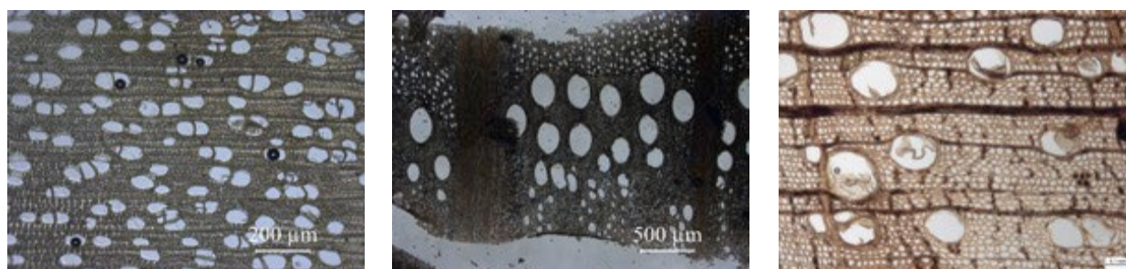
Fig. 4. Left, anatomical aspect of a diffuse porous wood (poplar). Middle, a semi-porous wood (walnut). Right, a ring porous wood (deciduous oak)
