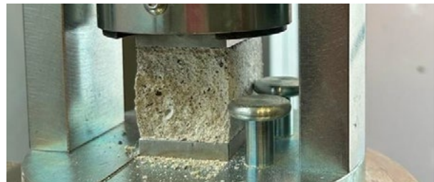
Fig. 4 Appearance of S3.5 after the compressive rupture
