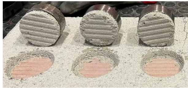
Fig. 6 Appearance of the S5 plaster after tearing: the observed failure is predominantly of the adhesive type.
