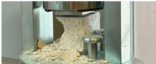
Fig. 3 Appearance of C3.5 after the compressive rupture.
