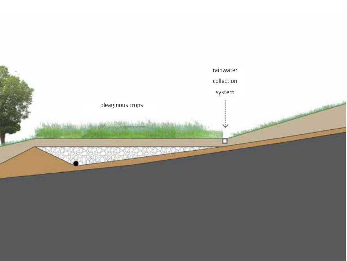
**Fig. 4** – Cross section of the landfill: The reshaped morphology of the landscape (graphics: Studio Arcoplan).
