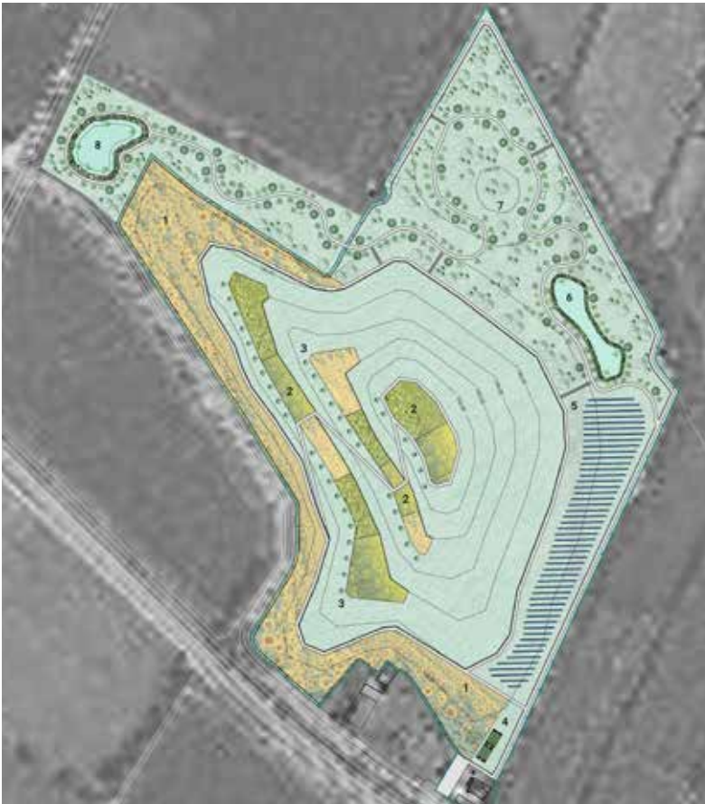
Fig. 11 – Plan of the requalification project: 1. Cultivation of sunflowers; 2. Cultivation of energy crops and phytoremediation meadows; 3. Lignocellulosic crops planted in rows; 4. Pilot phytoremediation plant; 5. Photovoltaic meadow; 6. Artificial lake for water collection; 7. Park (cycle tracks, footpaths, thematic itineraries, etc.); 8. Re-naturalised lake (graphics: Studio Arcoplan).
