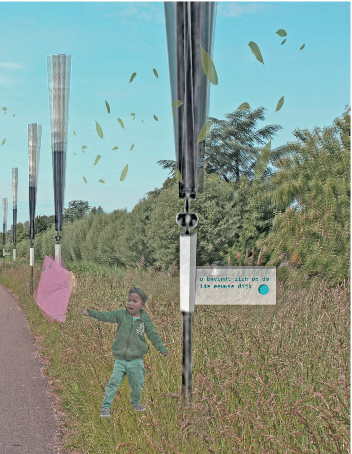
...s to a system of oscillating vertical axis wind turbines that while producing renewable energy indicate the dyke sign and the related age. ...llowing the IJ XIV century dyke (authors design concept elaboration).
