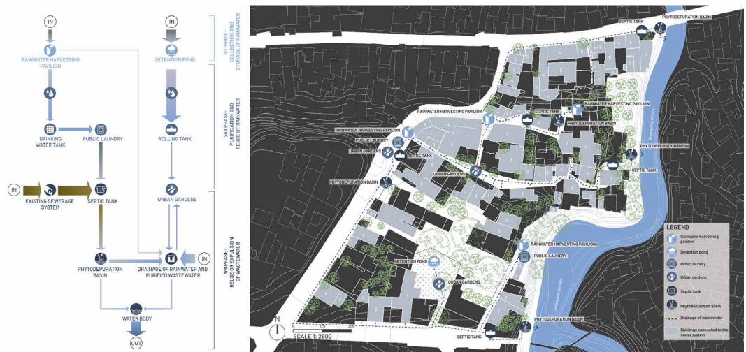
Fig. 6 - Sector F: hydraulic design strategy. Elaboration by the authors based on Rossignoli, L. (2022).
