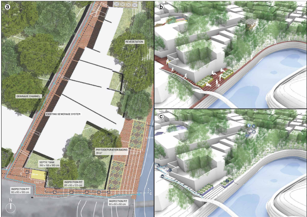
Fig. 10 – Sector F, third focus: the area along the Antequera stream. Masterplan (a), view of the project (b) and the connected water cycle (c). Elaboration by the authors based on Rossignoli, L. (2022).
