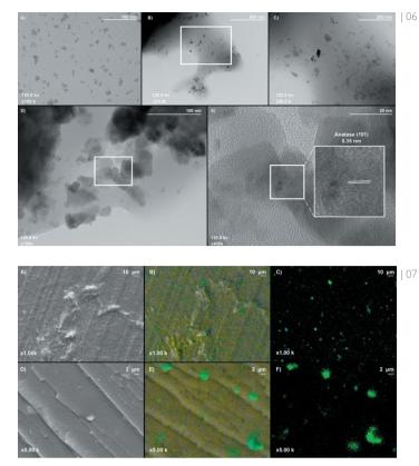
that they are present, along with an anatase structure of  $\text{TiO}_2$  nano-particles (Fig. 6E)
