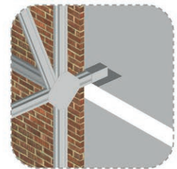
D. Slab to structure joint
