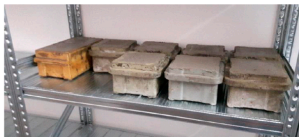
07 | Summary of the results of the tests carried out on 4 samples of concrete produced using cement (binder) and 0-4 mm recycled sand.
