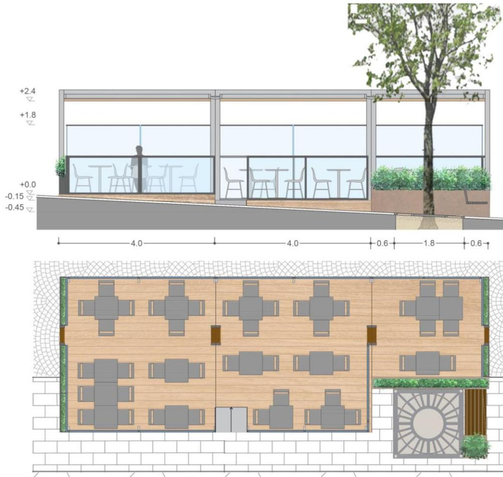
Figure 5 - plan and section view, metadesign of the dehors and public equipment modules on via Scarlatti. (elaboration by R. Mello).
