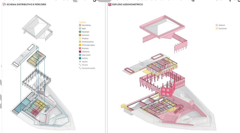
Fig. 05 Project proposal for the unfinished building to the north as the new secondary headquarters of XXXX of the ANBSC; distribution and composition scheme of the demolitions and additions; architectural drawings with evidence of the added parts and perspective views (Campagna, 2023).
