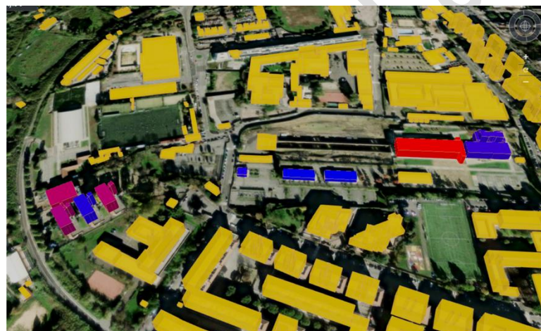
Fig. 5 – Execution in the 3D Web Map Client of a script for conditional coloring of a selection of Roma Tre University buildings, based on summer air conditioning power consumption (colors ranging from blue to red).
