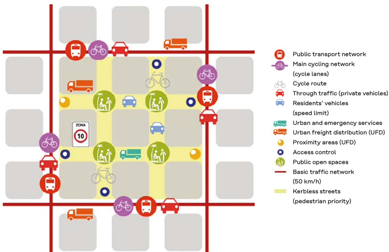
Fig. 01 – Diagram of a typical superblock in the final phase of implementation with all constituent parts, BCNecologia.
