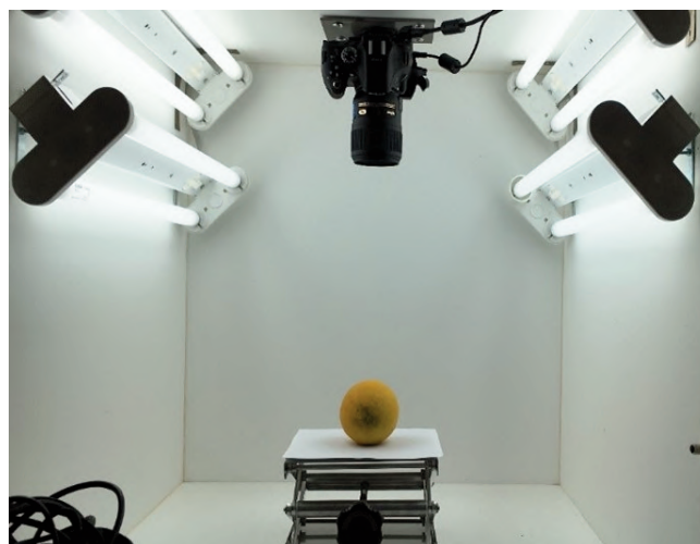
Fig. 1 - Bergamot RGB image acquisition using a laboratory inspection chamber equipped with a computer vision system.
