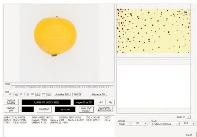
Fig. 2 - Bergamot colour determination through RGB image analysis.
